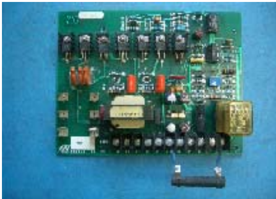
Figure 7: Top-view Photograph of the Constructed Converter.
