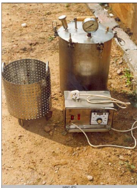
Figure 5: Aerial View of the Autoclave with the Inner Container (Olaoye, 2007).
