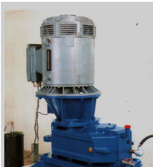
Figure12: SCHORCH Hydrogenerator 45KW, 400V, 1025rpm
