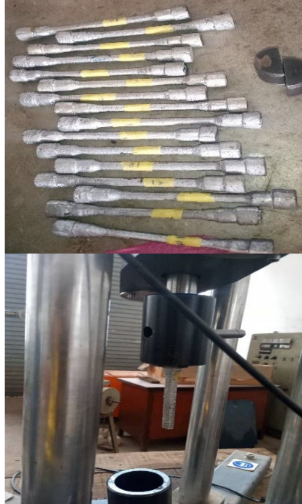
Figure 2: Produced Specimens for Tensile Strength Test.
