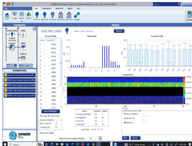
Figure 2: Daily Load Profile in the HOMER® PRO Software Interface.
