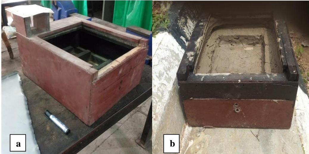
Plate 1: (a) Wooden Flat-Plate Solar Collector Housing and (b) Housing with Lining Material.
