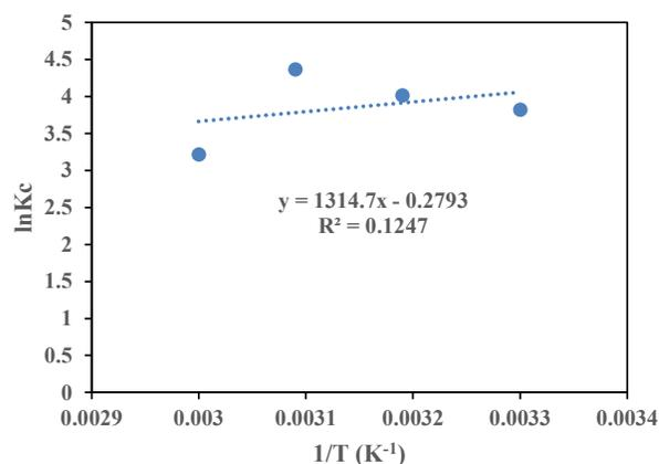
**Figure 12:** Plot of  $\ln K_c$  versus  $1/T$  for Thermodynamic Parameters of Pb (II) Adsorption onto NAC.
