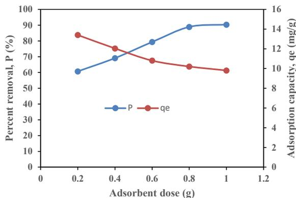
**Figure 5:** Effect of Adsorbent Dosage on Pb (II) Adsorption by NAC.
