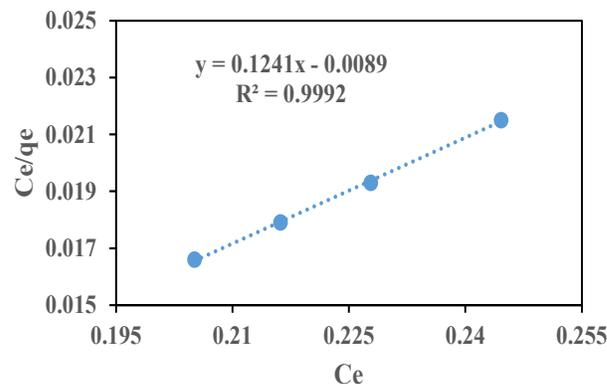
**Figure 8:** Langmuir Isotherm of Pb (II) onto NAC.
