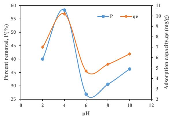
Figure 4: pH Effect on Pb (II) Adsorption by NAC.
