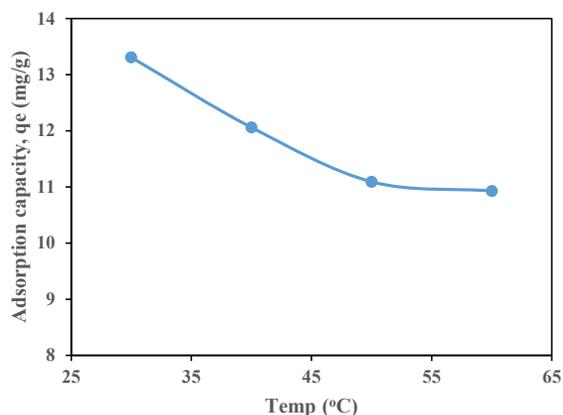
**Figure 7:** Effect of Temperature on Pb (II) Adsorption by NAC.
