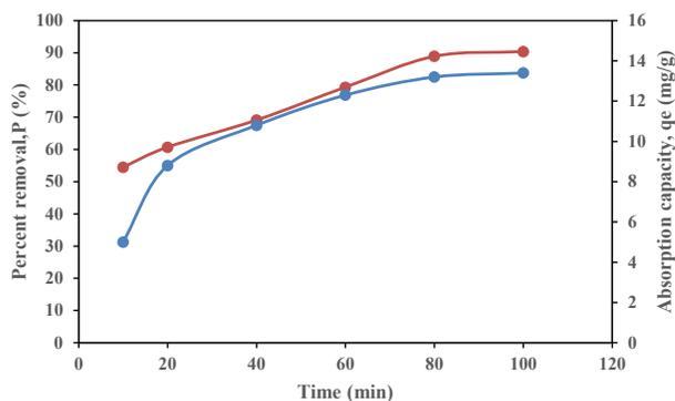
**Figure 6:** Effect of Contact Time on Pb (II) Adsorption onto NAC.
