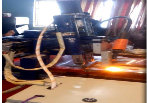
Figure 6: Developed Welding Mini-Robot in Operation.
