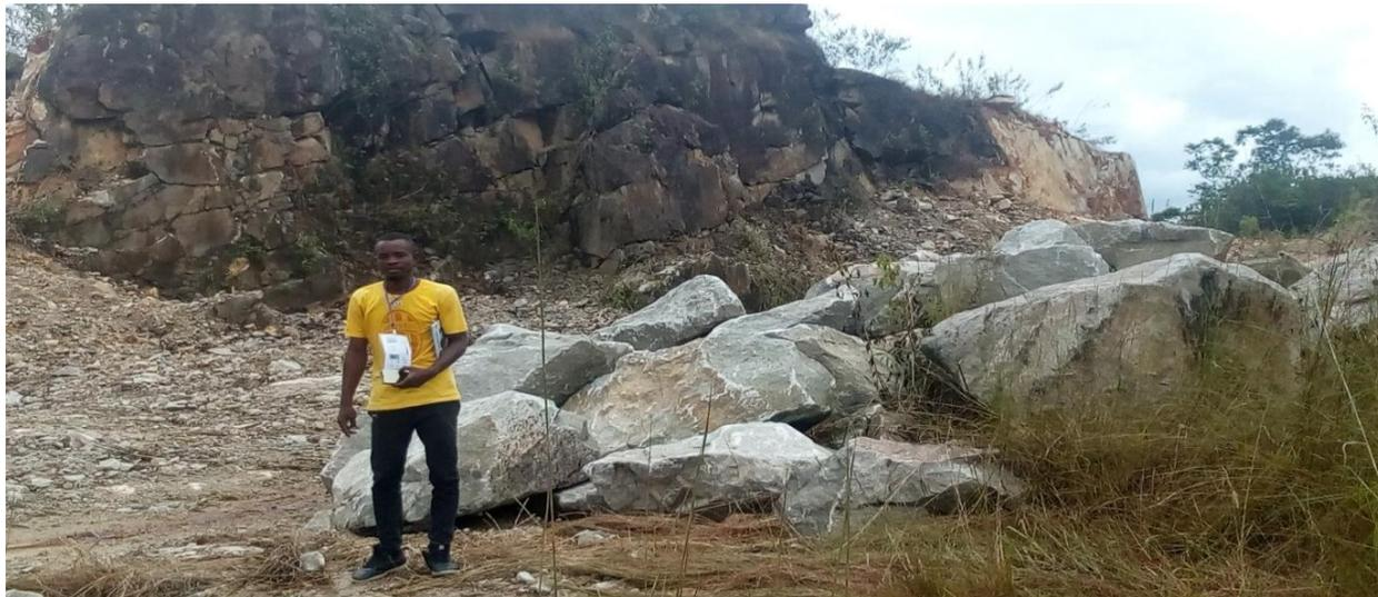
**Figure 3:** Field Photograph showing Fractures which have been Induced by the Blasting Vibrations at the Background and 1m and above Blasted Boulders at Nsan.
