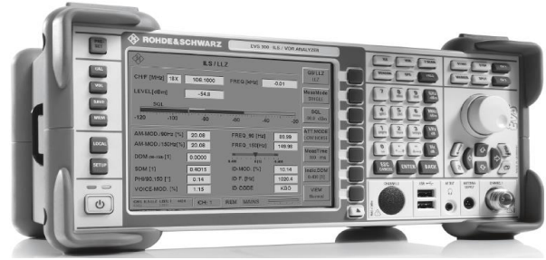
Figure 4: Picture of R&S EVS300 Analyzer (Rohde & Schwarz, 2014).
