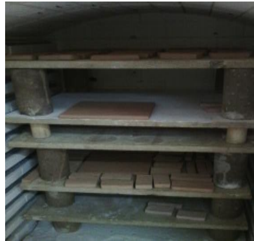
Plate I: Bisque Firing Test Pieces at Different Temperatures.
