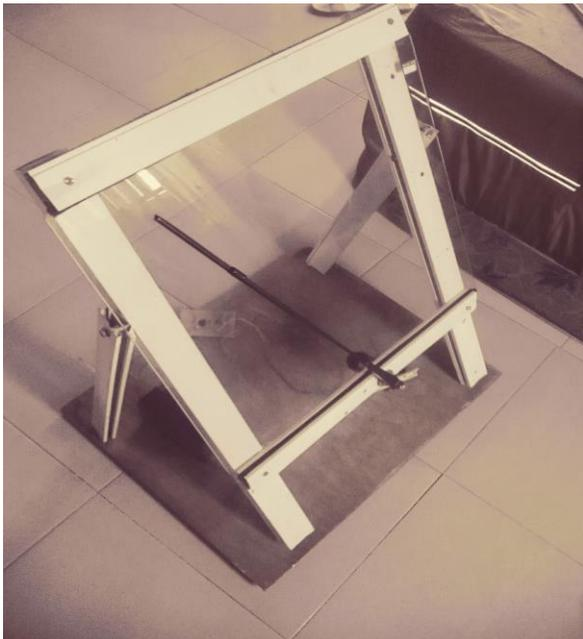
**Plate 7:** Automatic Rain Activated Wiper.
