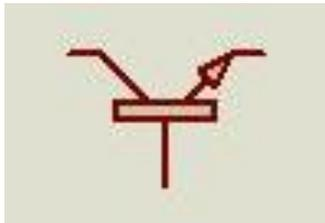
Figure 6: Transistor.
