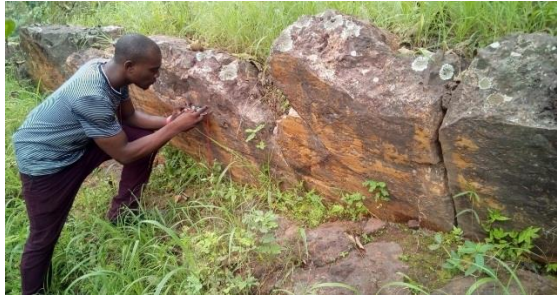
Plate 2: Field Photograph of Feldspathic Sandstone Hanging Wall or Right Hand of the Strike-Slip Fault showing Slickensides Surface and Joints Heave 25m and Throw 2.5m from the Footwall at Hilltop Area Abakaliki.
