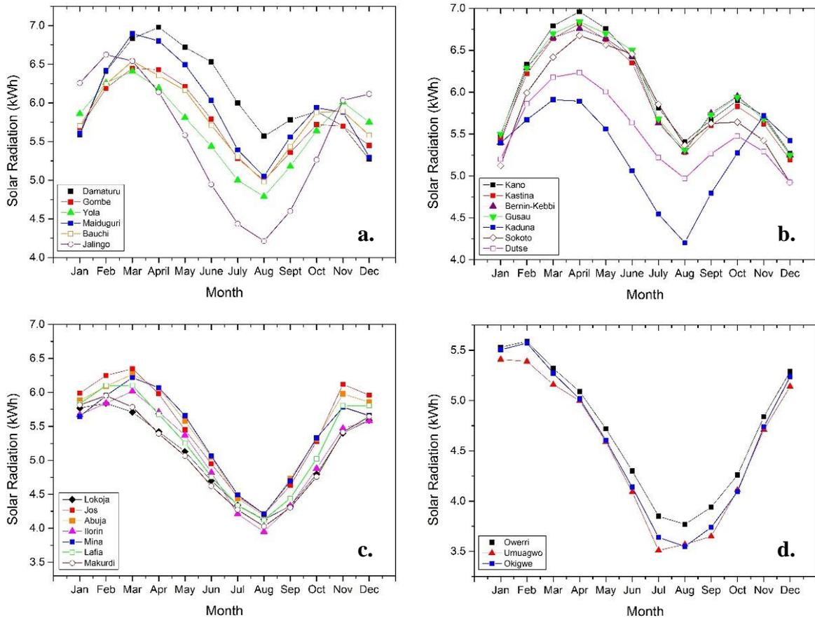
**Figure 2:** The Distribution of Average Monthly Solar Radiation Incident on the Horizontal Surface in Some Selected Locations in Nigeria.
