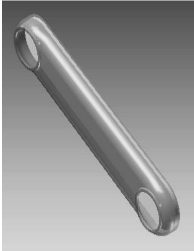
Figure 7: Model of Robot Arm Lower Arm and Cover.
