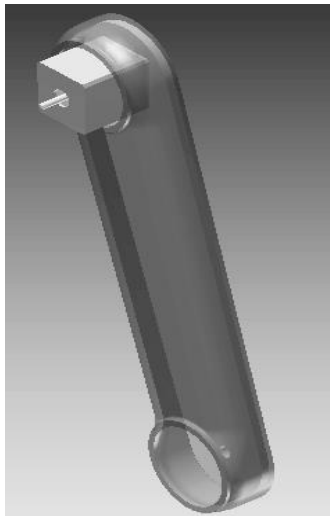
Figure 8: Model of Robot Arm's Upper Arm, Cover and Stepper Motor.
