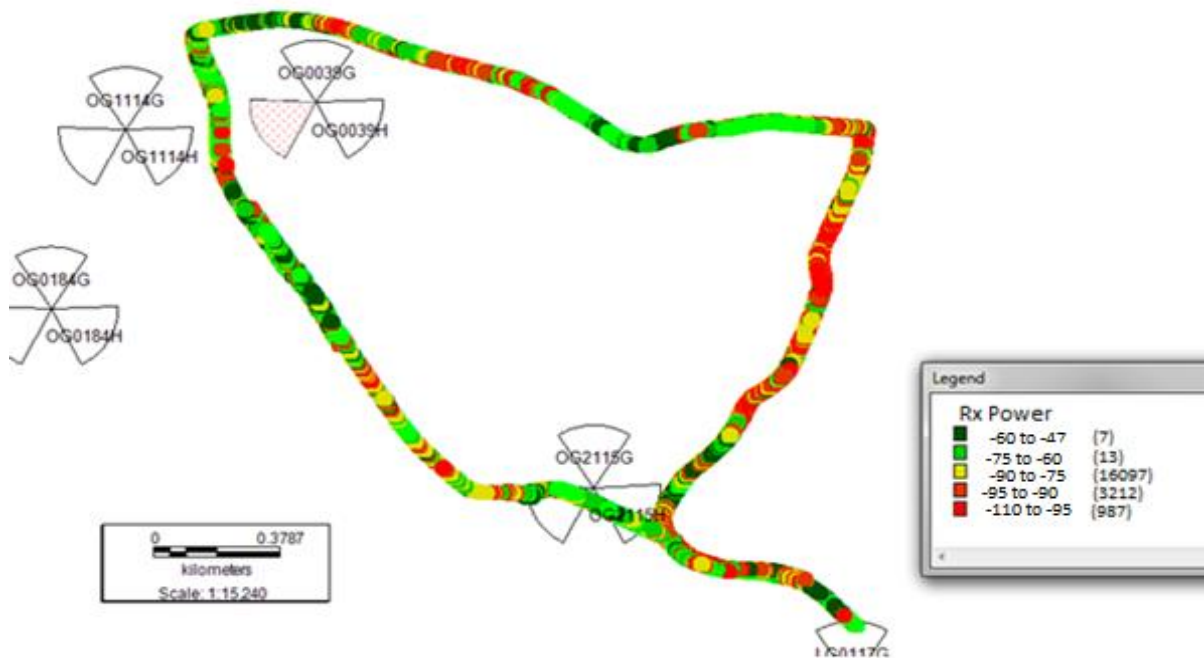
Figure 12: Screen Shot of Rx Power Result.
