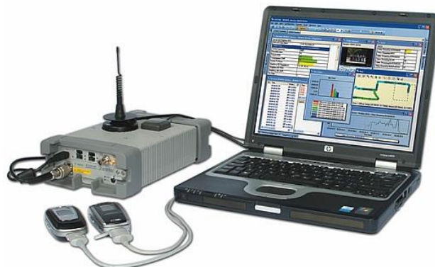
Figure 4: A Typical Drive Test Set-Up for Carrying Out Tests Using TEMS.
