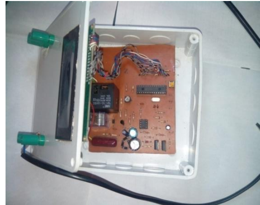
Figure 11: Internal View of the Digital Wattmeter.
