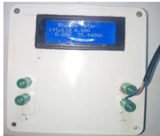
Figure 12: External View of the Digital Wattmeter.
