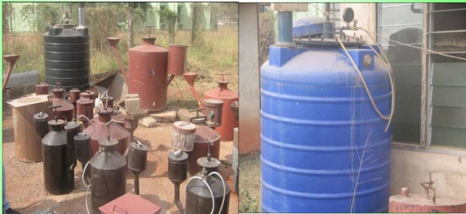
Figure 7: Sample of Household Biogas Digester – NCERD/.
