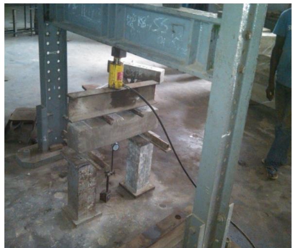
Figure 2: Testing Arrangement of Beam Specimens.
