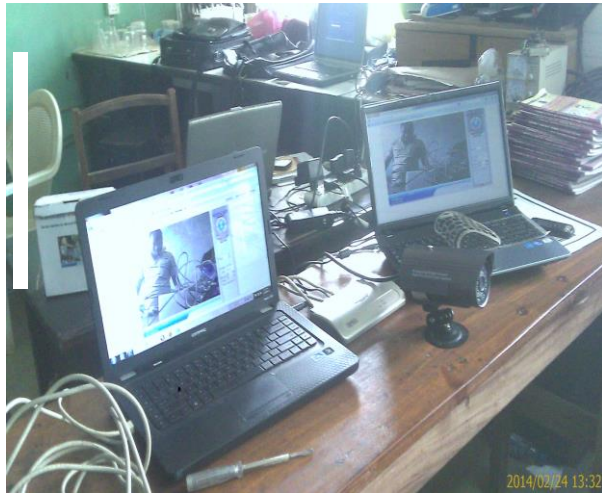
Figure 12: Connection and accessing the IP-Based Camera through 100MB/s Ethernet Switch.
