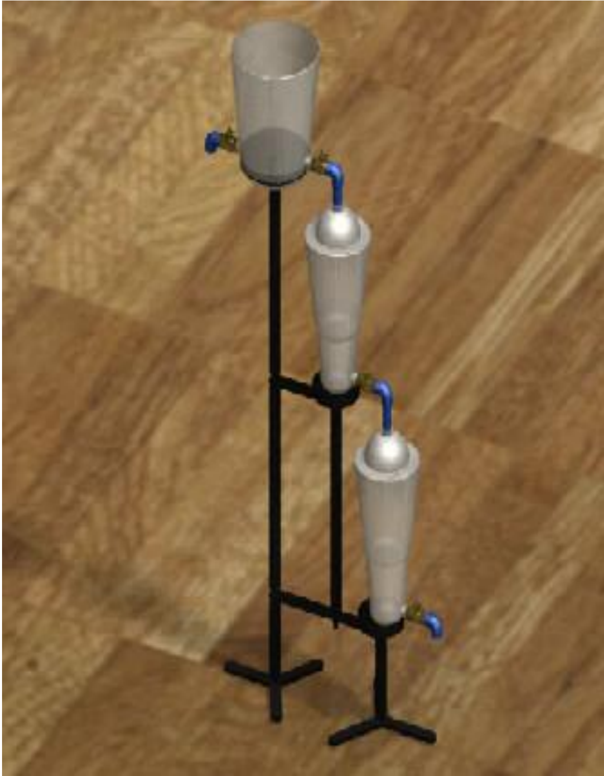
Figure 2: Pictorial View of De-Tottle Water Treatment Plant.
