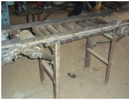
III: - Receiving Section, comprising the Rollers, Rollers' Rail, roller Hanger and the Jaw Joint Connector (link of the Second and the Third Sections).
