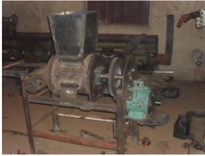
I:- fabricated processing section comprising the Hopper, milling chamber, nose-cone, electric motor, driven gear and the rigid stand. All these are from the scrap market
