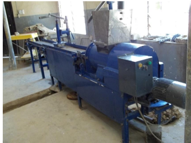
Figure 3: The Developed Tile Making Machine. (Source: Morakinyo, 2012 and Morakinyo et al., 2013).
