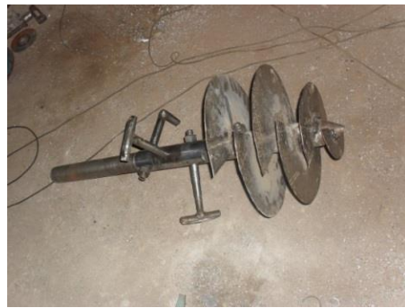
II: - Fabricated Shaft auger with milling paddles and blades.
