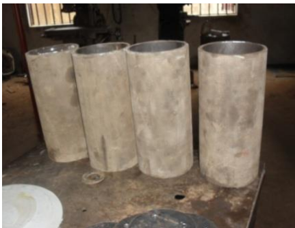
V:- Four cut Padded Cylindrical Pipes for the big conveyor rollers.
