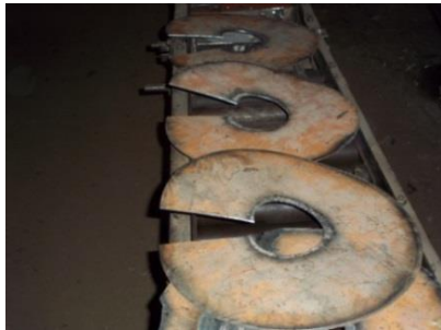
VI :- Cut And bended Auger Plates
