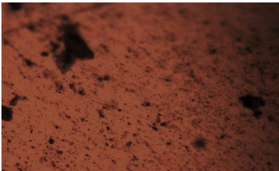
Plate 4: Photomicrograph of Zinc after Polishing with Superfine Polishing Cloth. Mag. X200.
