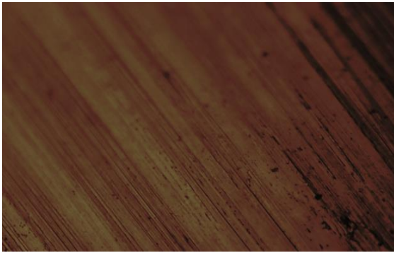
Plate 3: Photomicrograph of Zinc after Grinding with 60 microns Paper. Mag. X200.
