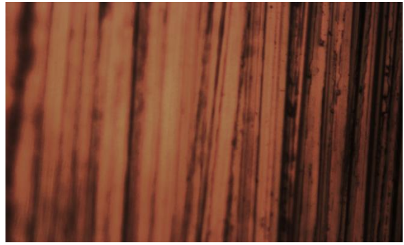
Plate 5: Photomicrograph of Steel after Grinding with 60 microns Paper. Mag. X200.
