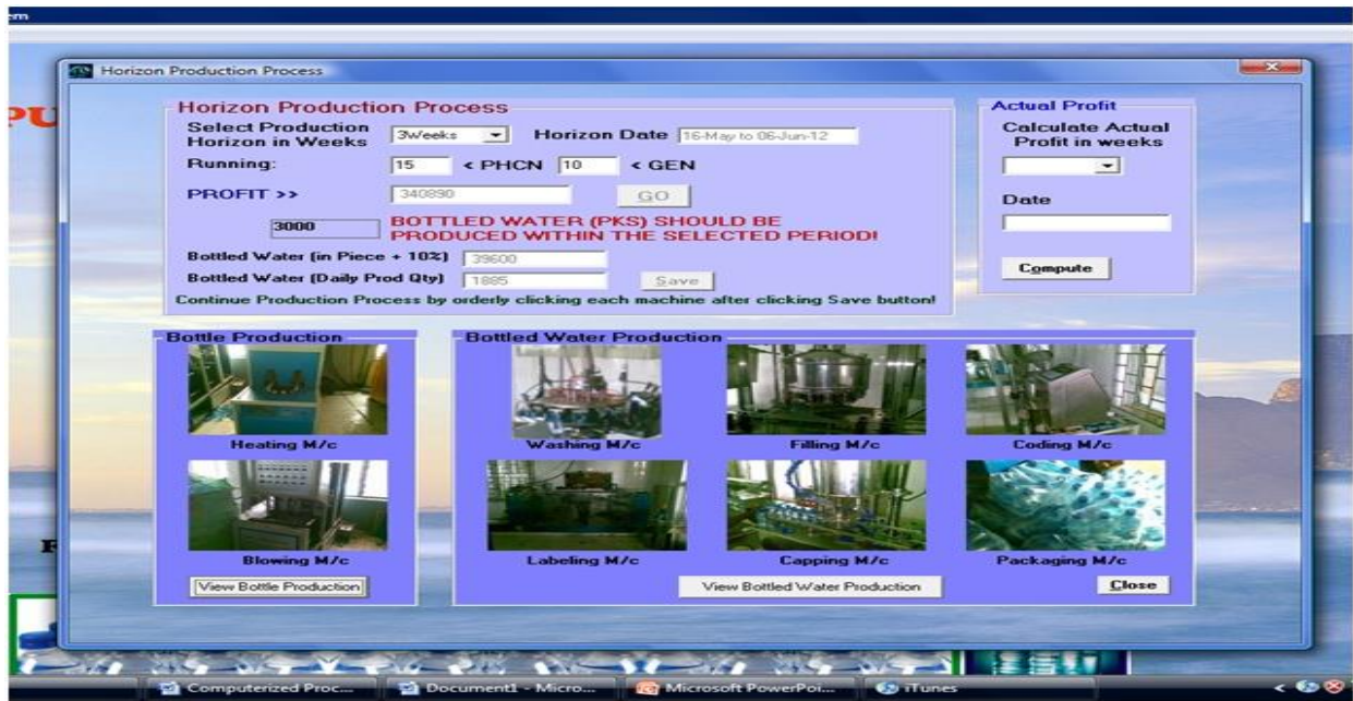
Plate 2: Horizon Production Process Module: Automatic Production Process Planning of all stored customer product demand quantity. The horizon periods are in weeks (1, 2, 3 or 4 Weeks) the developed software presenting the consistent lot size over the specified horizon period. (Extracted from developed software interface).
