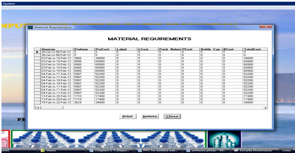
Plate 3: Material Requirement Module: Automatic Presentation of the raw material required quantity (preform, cap, label and pack nylon) and corresponding cost that would be required for the production process during the specified period of the process plan. (Extracted from developed software interface).
