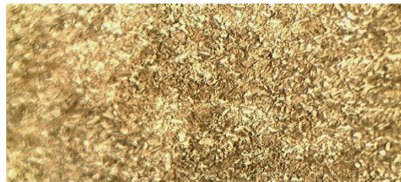
Plate 6: 80% Water + 20% alumino-silicate quenched microstructure of 0.33%C Steel showing fewer Martensite in higher proportion of untransformed Austenite. Etched in 2% Nital. Magnification x 400.
