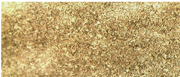
Plate 3: 95% water + 5% alumino-silicate quenched microstructure of 0.33%C Steel showing high proportion of full lath Martensite. Etched in 2% Nital. Magnification x 400.
