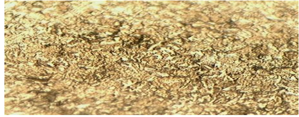
Plate 4: 90% water + 10% alumino-silicate quenched microstructure of 0.33%C Steel showing Martensite and low proportion of untransformed Austenite. Etched in 2% Nital. Magnification x 400.
