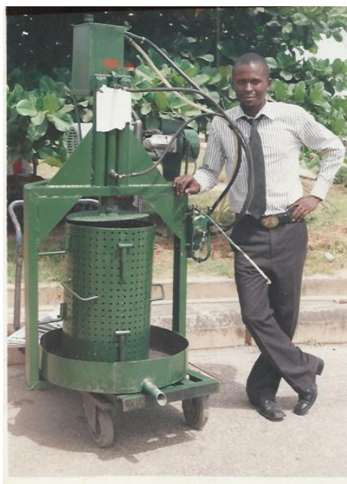
Figure 3: Designed and Fabricated Motorized Hydraulically Operated Palm Oil Press with the Designer Beside it.
