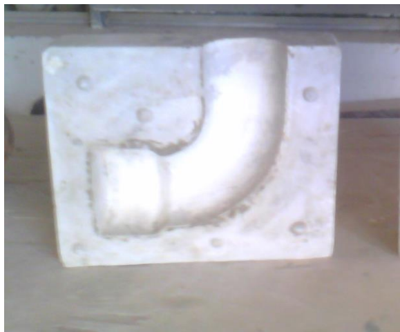
Plate 2: Elbow pipe in the mold (half of the mold removed to allow clay pipe to dry).
