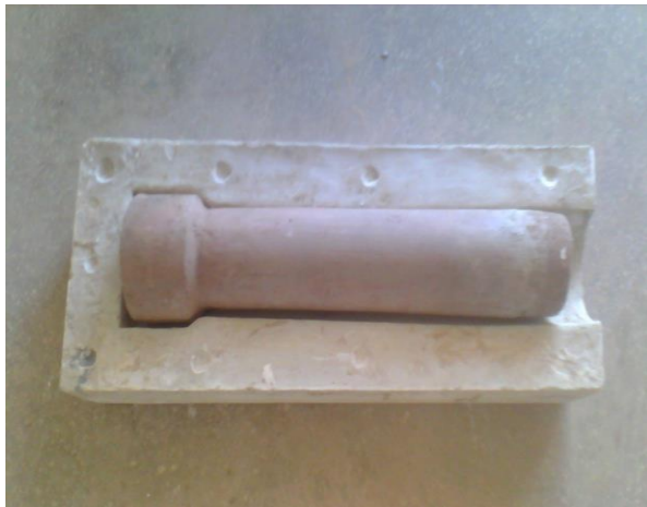
Plate1: Linear pipe in the mold (half of the mold removed to allow clay pipe to dry).
