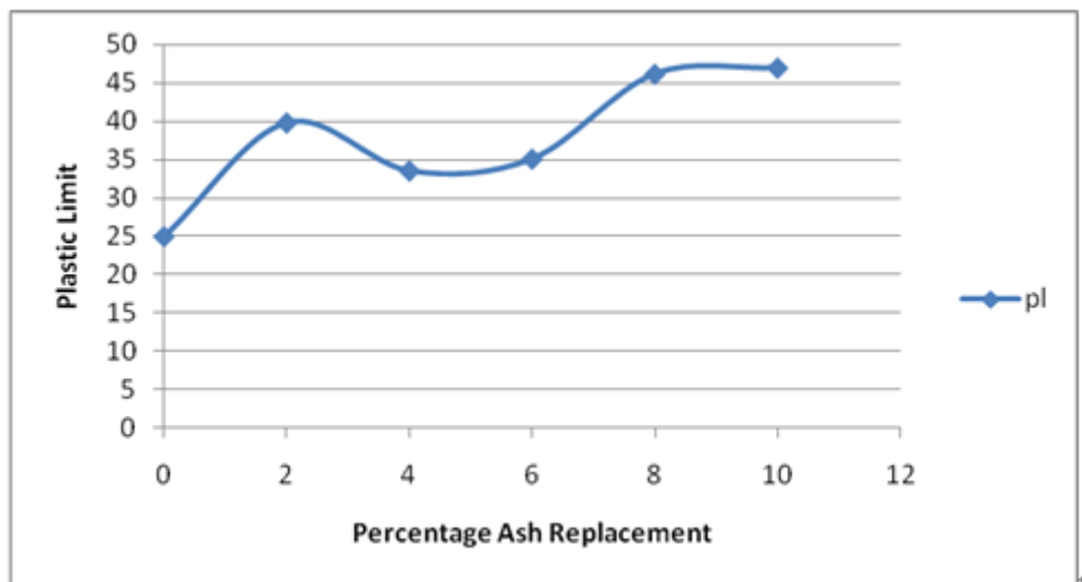
Figure 3: Relationship between Plastic Limit and Percentages of Ash Replacement.
