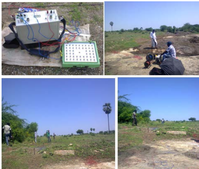
Figure 2: The 2D ERI Field Survey carried out in the Granitic Terrain.
