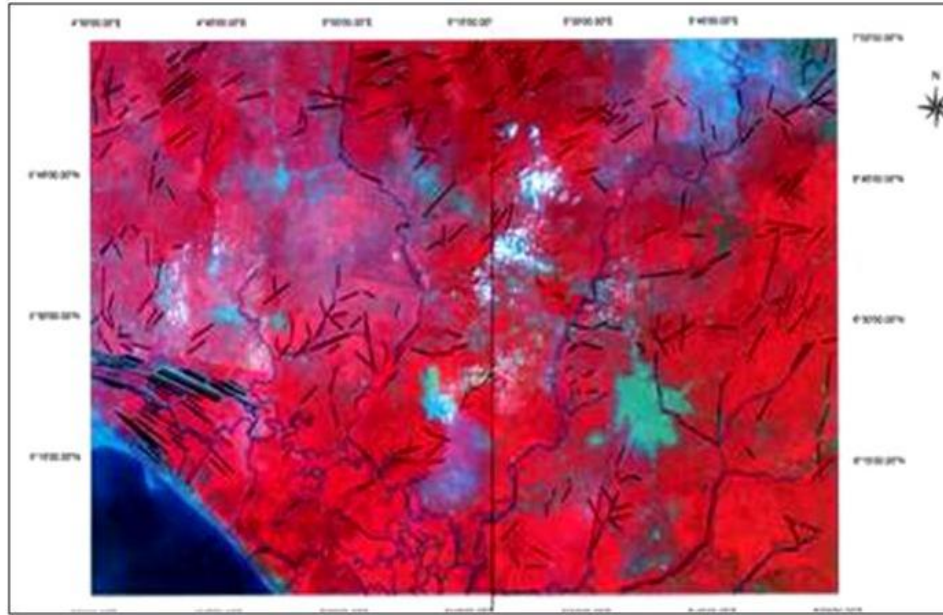
Figure 7a: Landsat – ETM Image of the Study Area Showing Interpreted Lineaments and Drainage.
