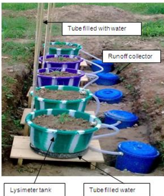
Plate 1: Typical Setup of the Mini-Lysimeter.
