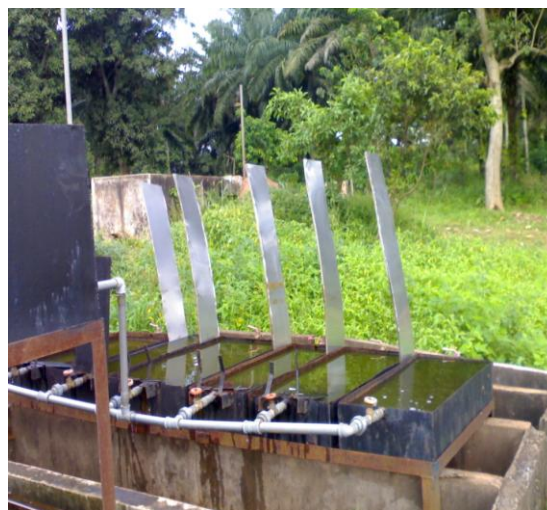
Figure 2: Right Position of Reflectors.
