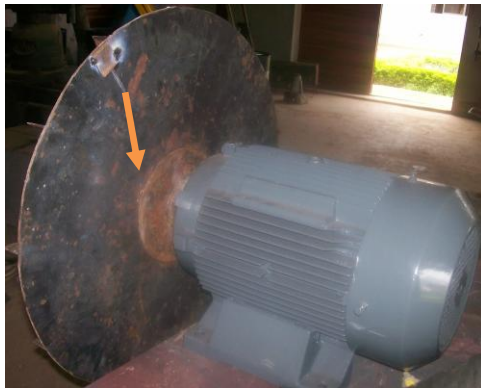
Plate 8: Out-of-Balance Mass added for Impeller Dynamic Balance.
