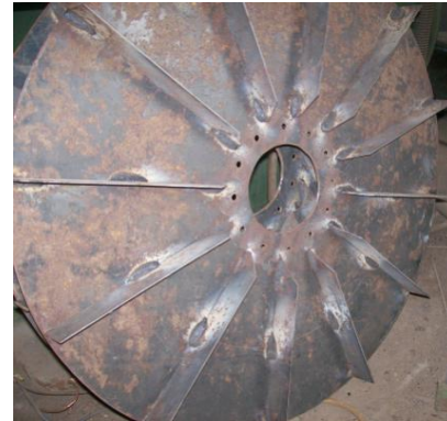
Plate 3: Radial Impeller under Construction.
