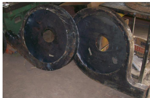
Plate 6: Clockwise and Anti-Clockwise Volute Casings under Construction.
