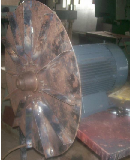
Plate 7: Radial Impeller undergoing Dynamic Balancing.
