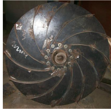
Plate 2: Backward Curved Impeller under Construction.
