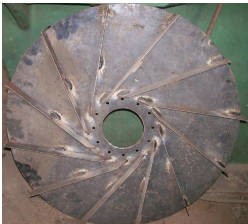
Plate 1: Forward-Inclined Impeller under Construction.
