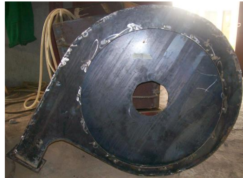
Plate 5: Anti-Clockwise Volute Casing under Construction.
