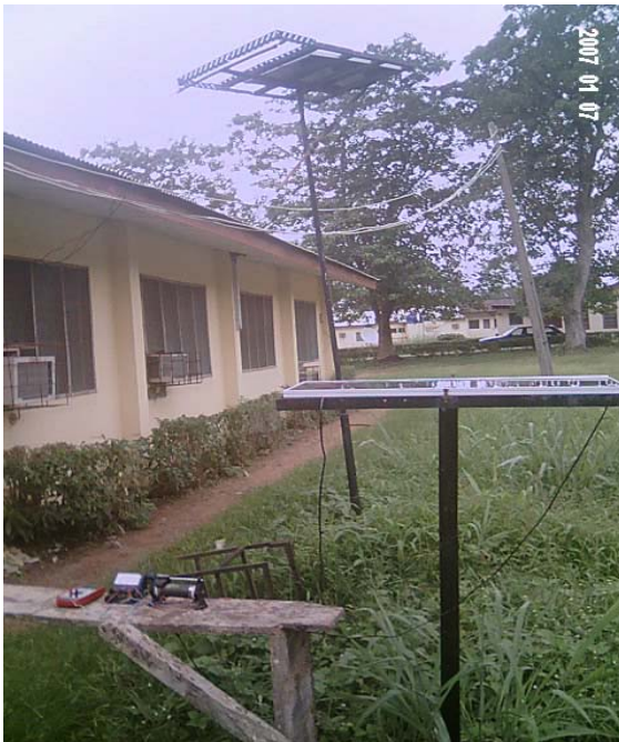
Figure 2: The Prototype of Solar Array of Test and Control ASPS.
