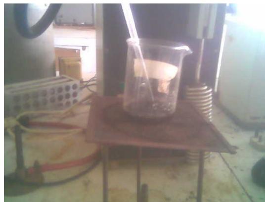
Plate 1: Grease Production Set-up.
