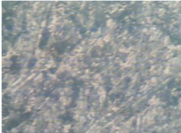
Plate 2: Immersed SEM 0.6mm of Al, Mx400, 2% Nitric acid and 98% Ethyl Alcohol.
