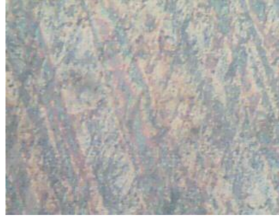
Plate 4: Immersed SEM 1.2mm of Al, Mx400, 2% Nitric acid and 98% Ethyl Alcohol.
