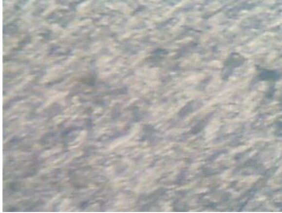
Plate 1: Initial state of SEM 0.6mm Al, Mx400, 2% Nitric acid and 98% Ethyl Alcohol.
