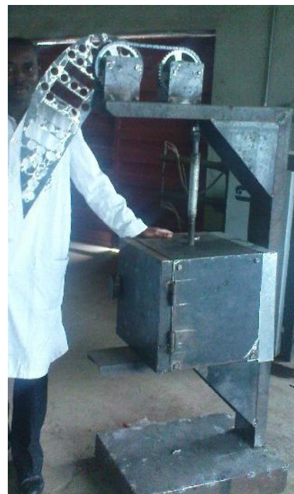
Figure 7: The Developed Constant Stress Creep Testing Equipment.
