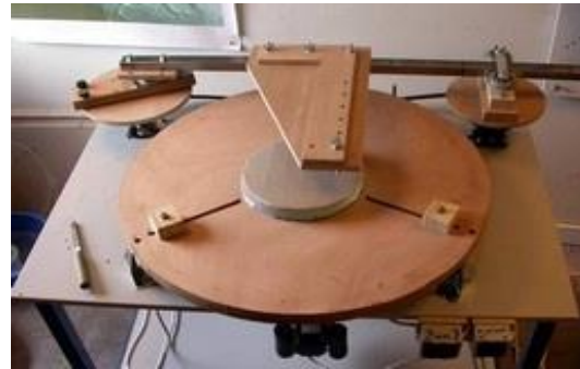
Figure 6: Jean-Marc Leclaire's Polishing Machine (Source: Jean Texereau, 1958)
