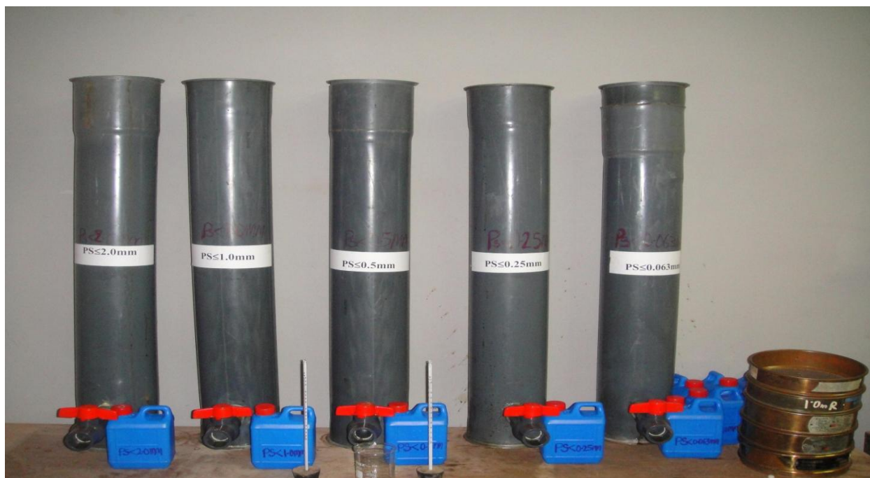
Figure 1: Constructed PVC Simulation Columns, Sampling Cans, Five Canadian Standard Wire Screen Sieves, Thermometers and 250mL Beaker.
