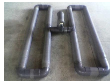
Figure 4: Pipes for Flotation.
