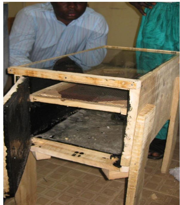
Figure 5: Direct Mode Solar Dryer.
