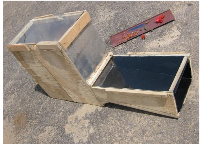
Figure 4: Mixed Mode Solar Dryer.
