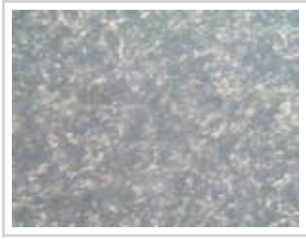
Plate 1: 0.9mm Aluminum Sample (Un-soaked), X400, 2% Nitric Acid and 98% Ethyl Alcohol.
