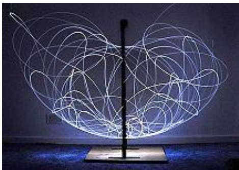
Figure 3: Double Pendulum Tracked with LED Light.
