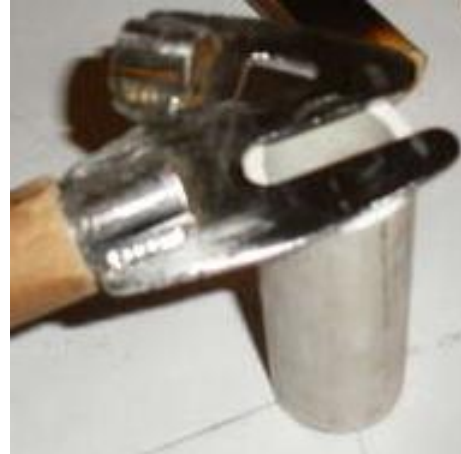
Figure 2: Dropout Showing Jig Design.
