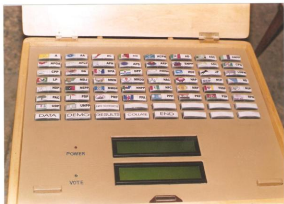
Figure 4: Picture of EVM Unit Showing Party/Function Buttons and LCD Display Modules.
