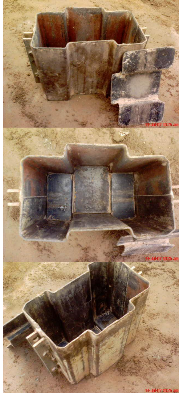
Figure 1: Locally Fabricated Steel Mould
