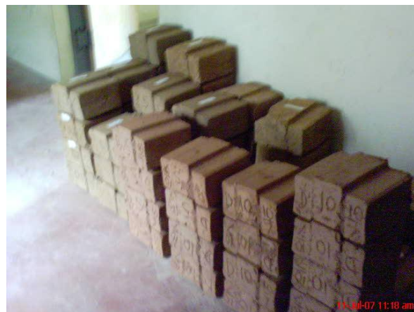
Figure 2: Stacking of Lateritic Interlocking Blocks.
