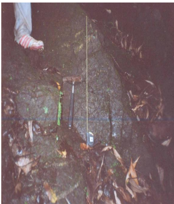
Figure 14: Fault and Fractures at Kekibe Hills. Normal Fault Throw 70cm, 40cm, 30cm in Granulitic Rocks.
