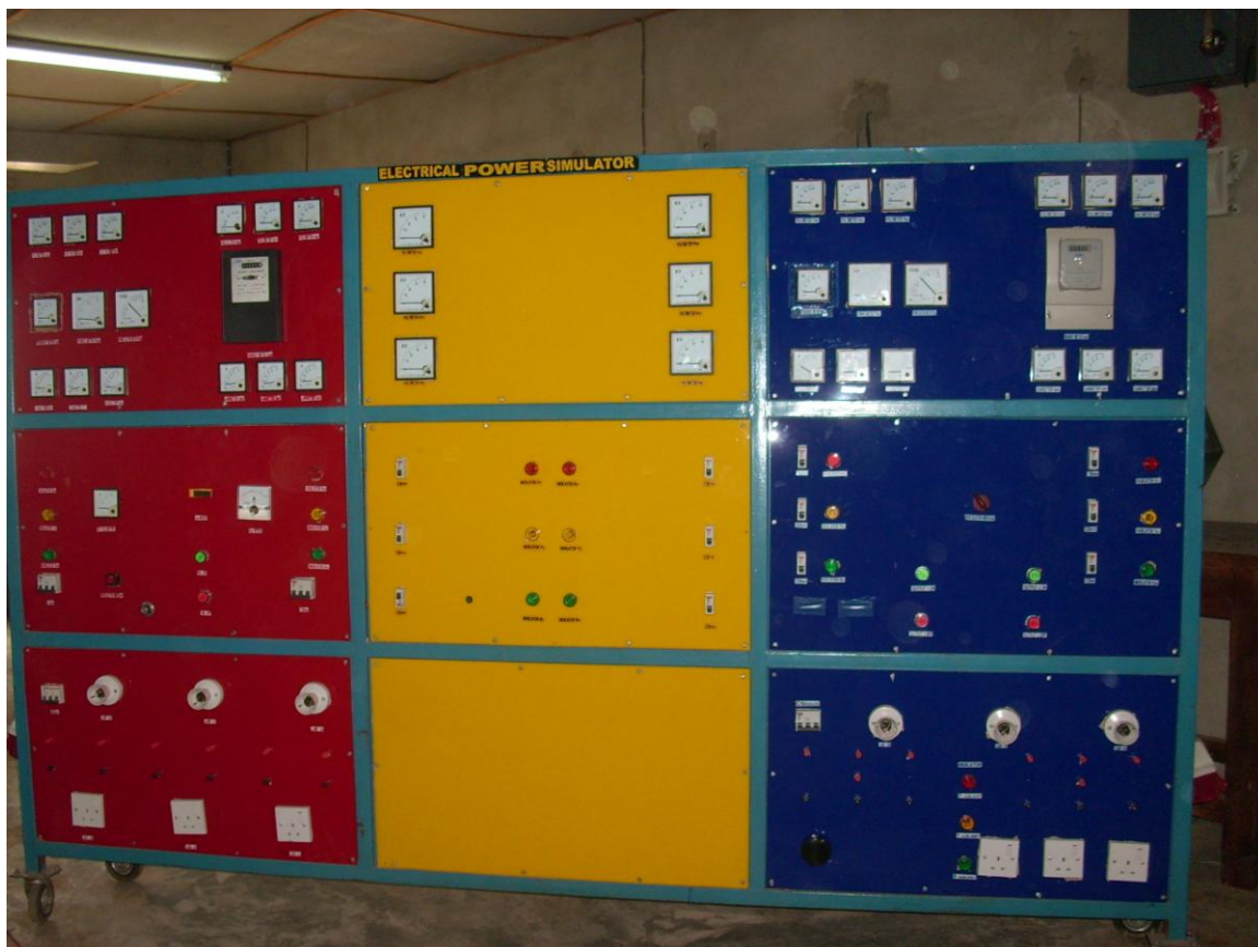
Figure 2: Power System Simulator (PSS): A Self-Contained Unit, which Simulates all Parts of the Electrical Power Network and their Protection, from Generation to Utilization points.
