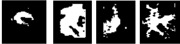
Figure 2: Isolation of Some of the Pores in Oil and Water Quenched Microstructures of Al-20%wtMg.
