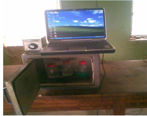
Figure 1: The Constructed Furnace for Thin Film Annealing.
